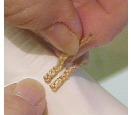
Apply glue to the next channel, and place the next braid.
