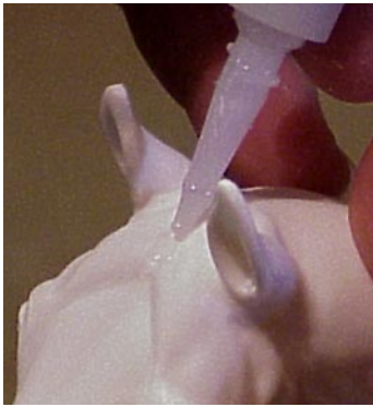
Apply a little super glue into the lower part of the channel only.
